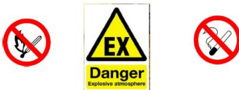
Figure 15 Signs of flammable material - Examples
